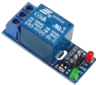
♦ MODULO RELAY 1 CANAL ♦ RELAY 5V ♦ CONDUCCION 250VAC 10A
