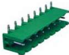
♦ TERMINAL BLOCK 8P CURVO ♦ PITCH 5.08mm ♦ 300V 15A MAX
