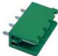
♦ TERMINAL BLOCK 4P RECTO ♦ PITCH 5.08mm ♦ 300V 15A MAX
