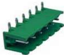
♦ TERMINAL BLOCK 6P CURVO ♦ PITCH 5.08mm ♦ 300V 15A MAX
